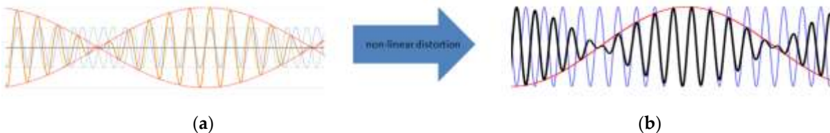
Figure 2. A non linear distortion happening inside a non-linear medium can generate a perceivable signal of the non-linear frequencies: (a) out of the beating between f_1 and f_2 under the influence of a non-linear distortion in the medium can emerge (b) the non-linear frequencies: The sum-frequency (f_1 + f_2) (dark blue) and the difference frequency (f_1 - f_2) (red) modulating its envelope. The modulated frequency (f_1 + f_2) is the carrier frequency of the modulating frequency. The Fourier transform contains only the two nonlinear frequencies (f_1 + f_2) and (f_1 - f_2) .
