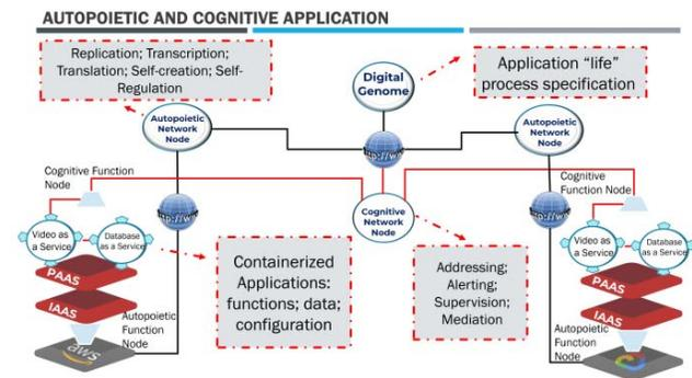
Figure 2: A structural machine framework deploying a self-managing video service application in a multi-cloud network.
